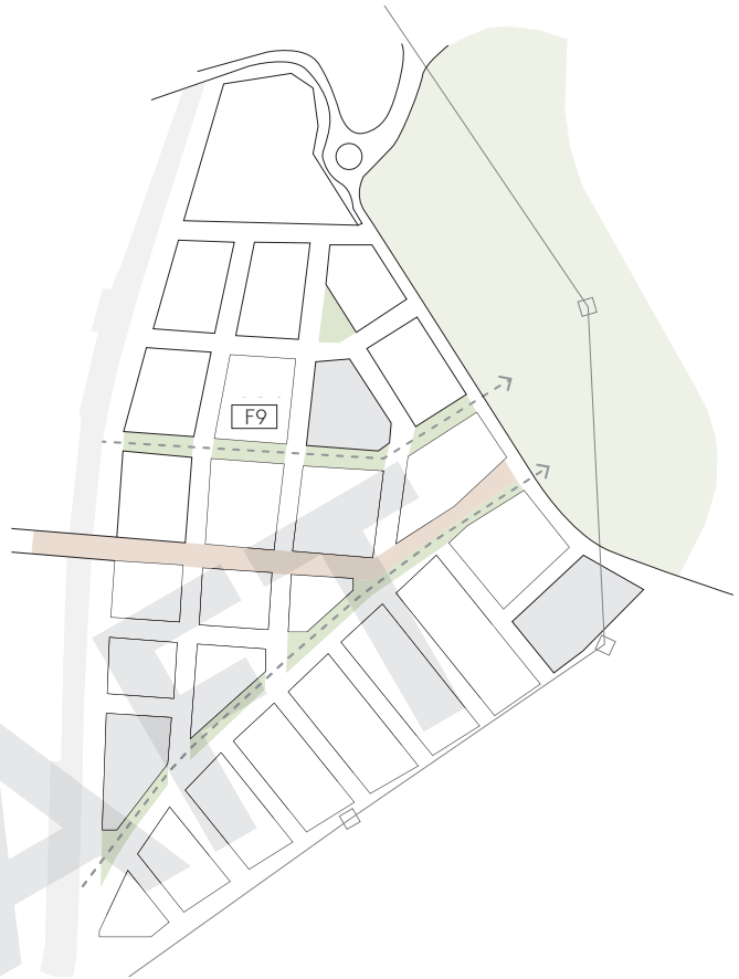
Fig 126. The flood relief embedded within indicative masterplan plot layout
